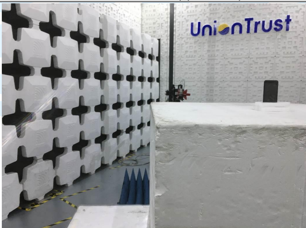
Radiated emission Test Setup (Above 1 GHz)
