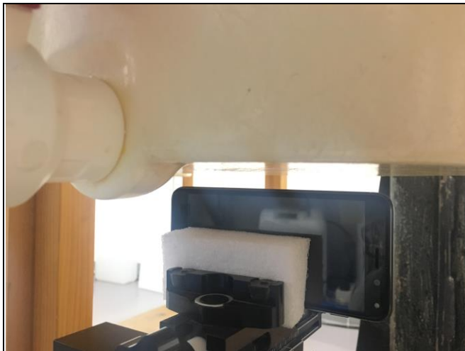
Left Side of EUT with 1.0 cm Gap
