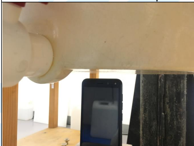
Top Side of EUT with 1.0 cm Gap
