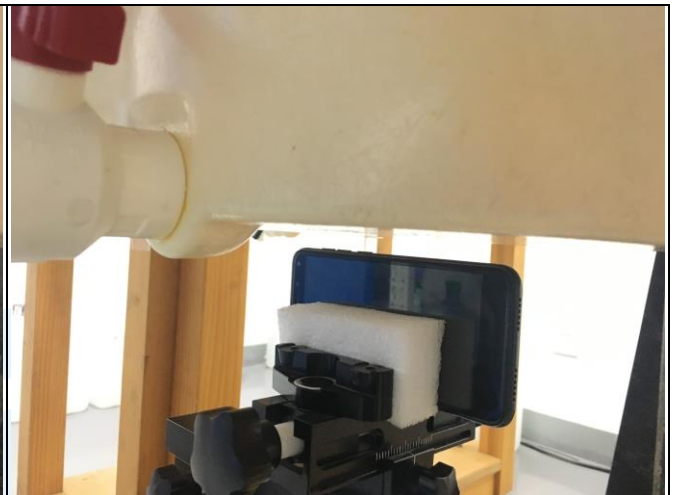
Right Side of EUT with 1.0 cm Gap
