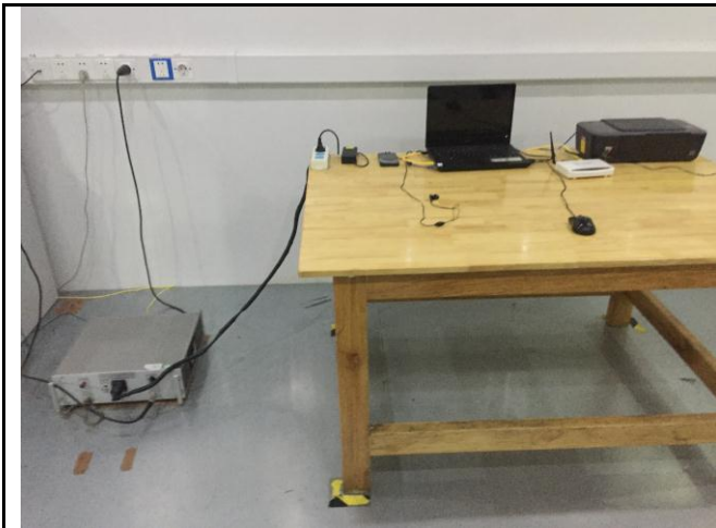
Conducted Emissions Test Setup – Front View
