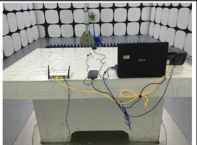
Radiated Emissions Test Setup Above 1GHz
