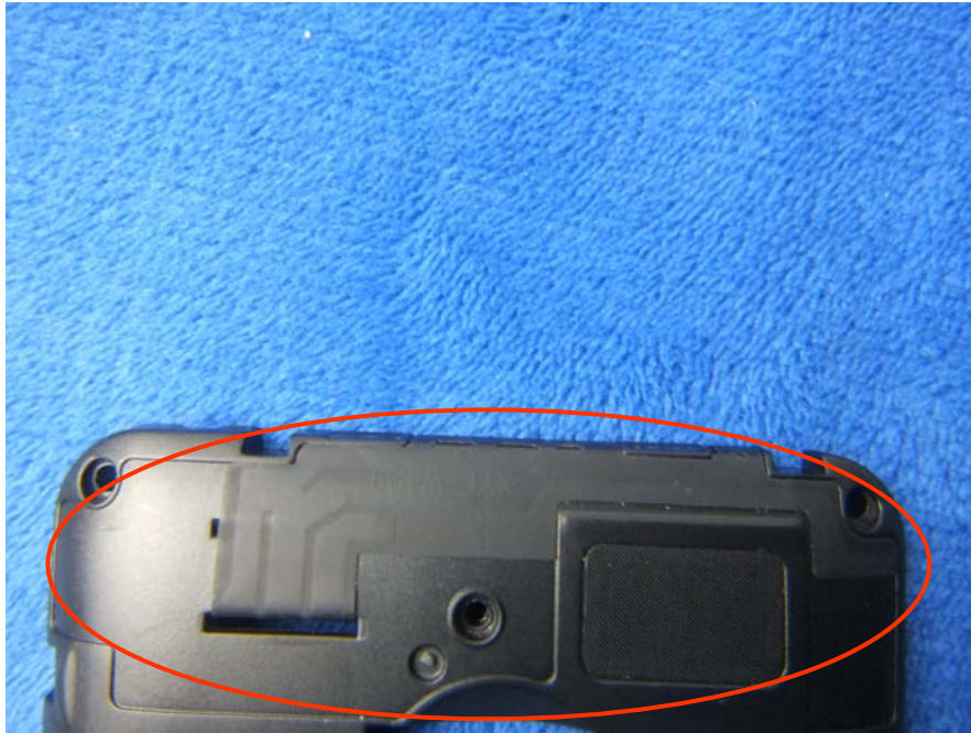
GSM/PCS/UMTS-FDD Antenna View
