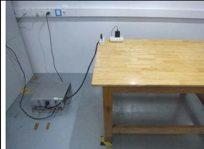
Conducted Emissions Test Setup Front View
