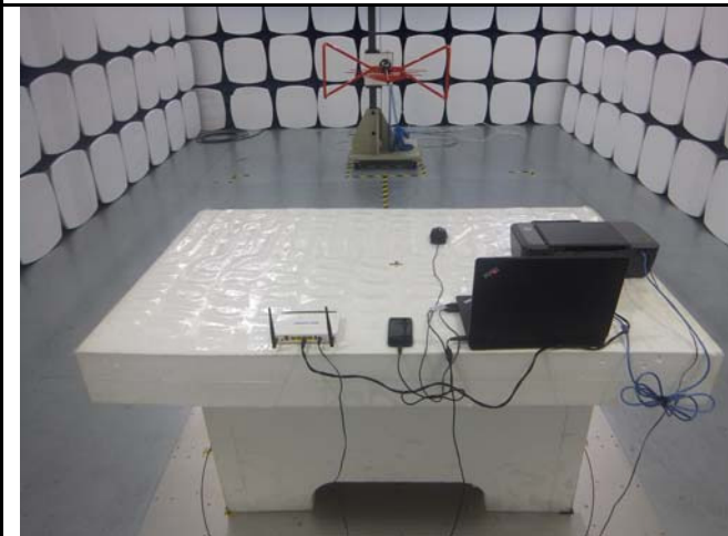
Radiated Emissions Test Setup Below 1GHz
