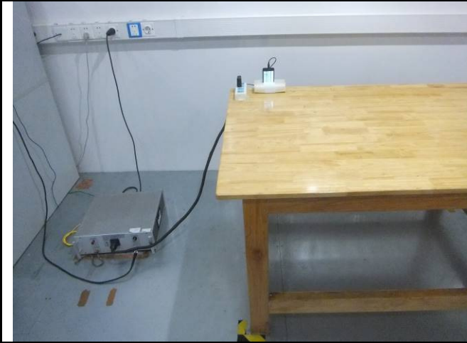
Conducted Emissions Test Setup Front View
