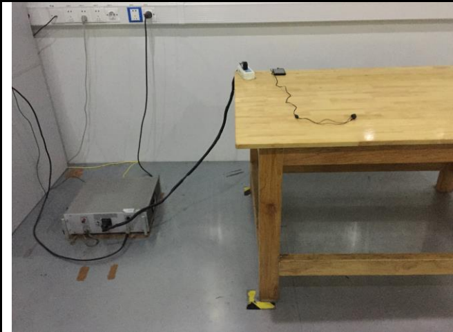
Conducted Emissions Test Setup Front View
