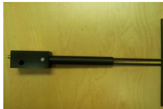
Figure 1 – MVG COMOSAR Validation Dipole
