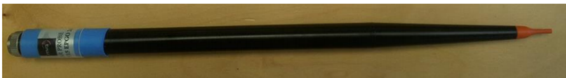
Figure 1 – MVG COMOSAR Dosimetric E field Dipole
