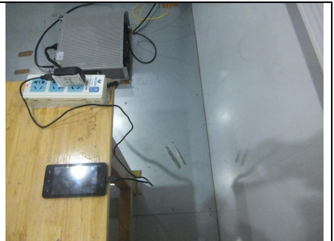
Conducted Emissions Test Setup Side View
