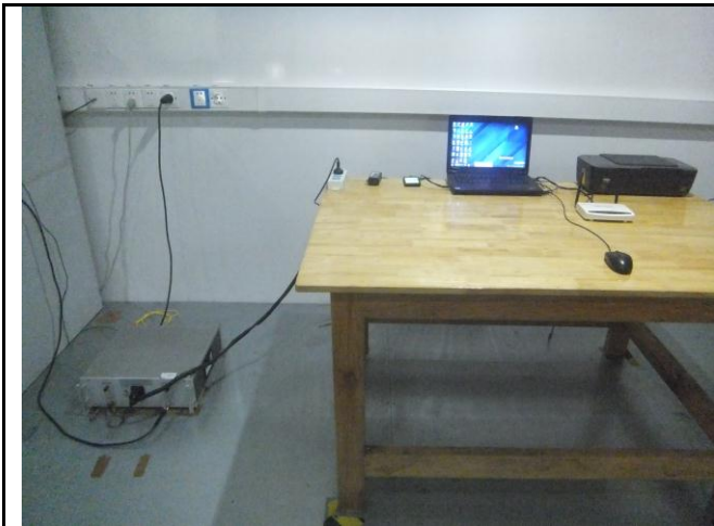
Conducted Emissions Test Setup – Front View
