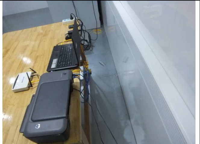
Conducted Emissions Test Setup – Side View
