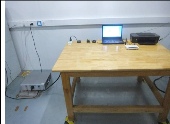
Conducted Emissions Test Setup – Front View
