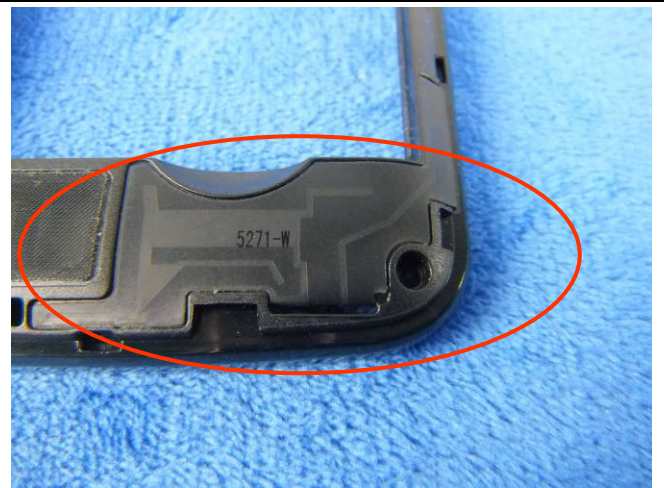
GSM/PCS/UMTS-FDD - Antenna View
