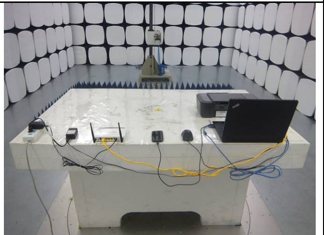
Radiated Spurious Emissions Test Setup Above 1GHz
