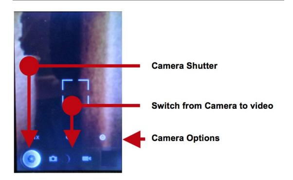
You may adjust various settings for the camera by pressing the camera options while in the camera interface.
