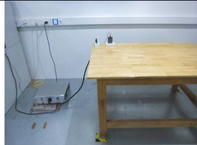
Conducted Emissions Test Setup Front View
