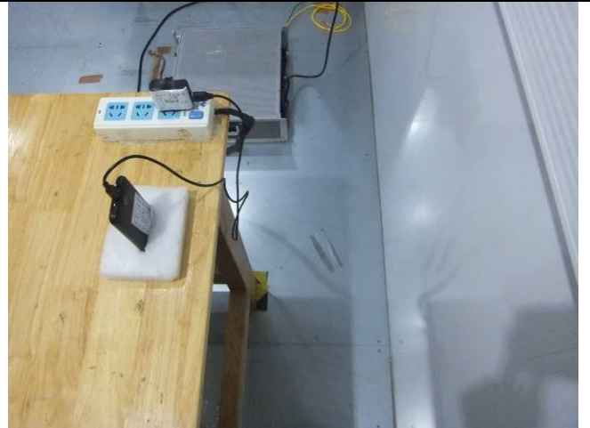
Conducted Emissions Test Setup Side View
