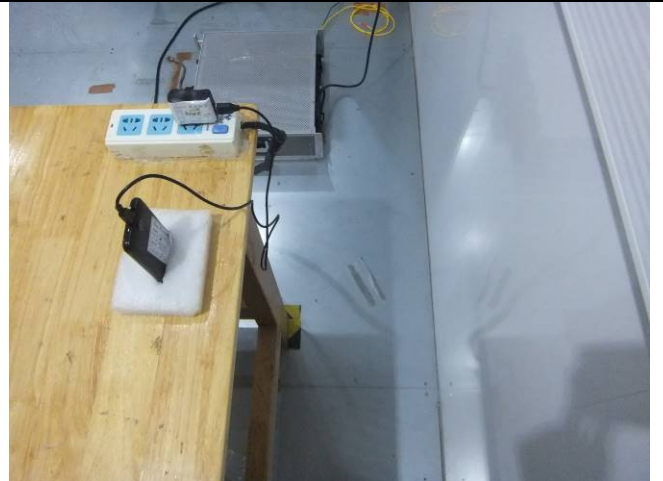
Conducted Emissions Test Setup Side View
