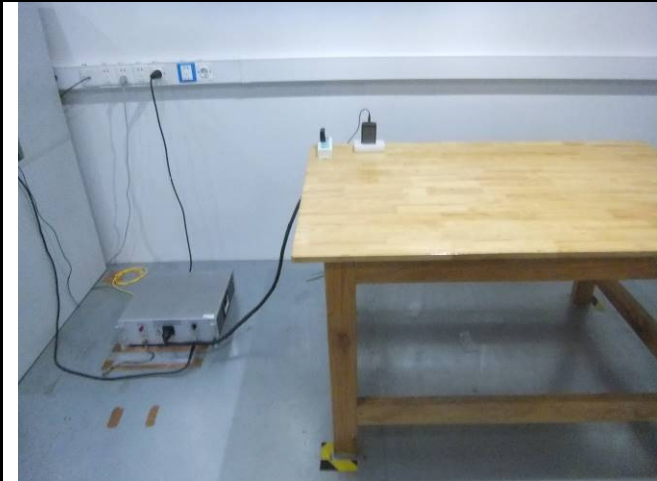
Conducted Emissions Test Setup Front View
