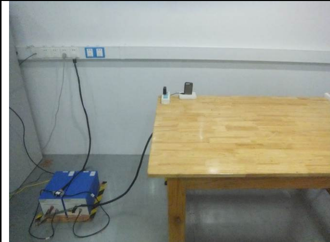
Conducted Emissions Test Setup Front View
