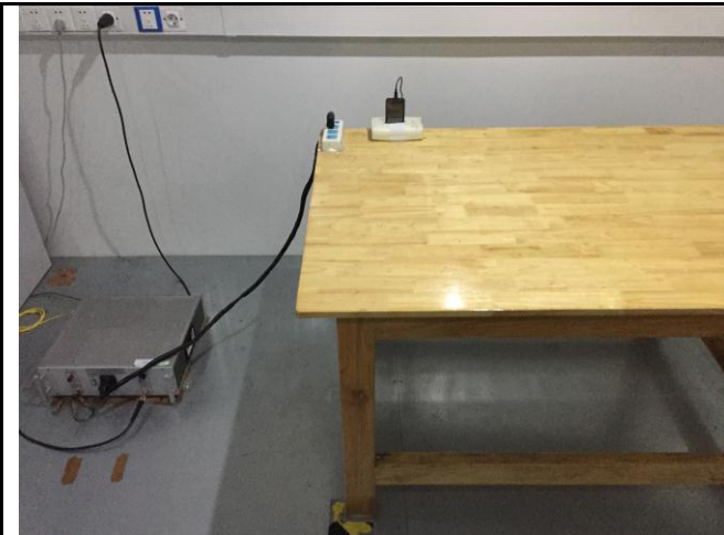
Conducted Emissions Test Setup Front View
