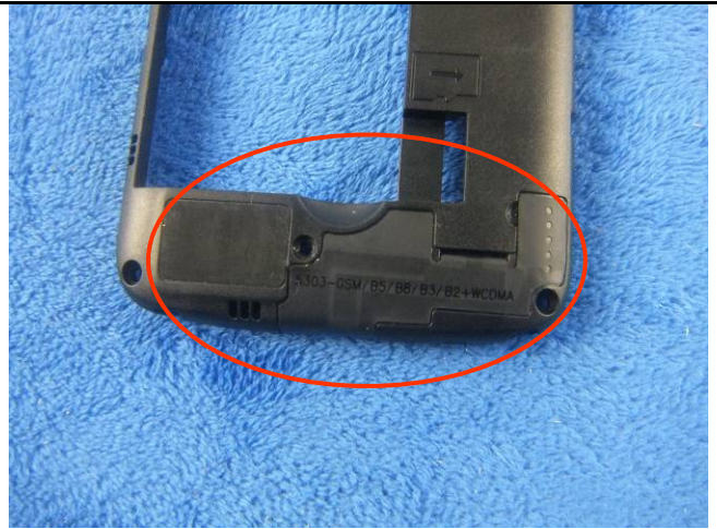
GSM/PCS/UMTS-FDD Antenna View
