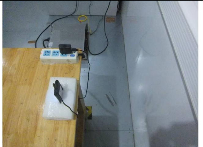
Conducted Emissions Test Setup Side View
