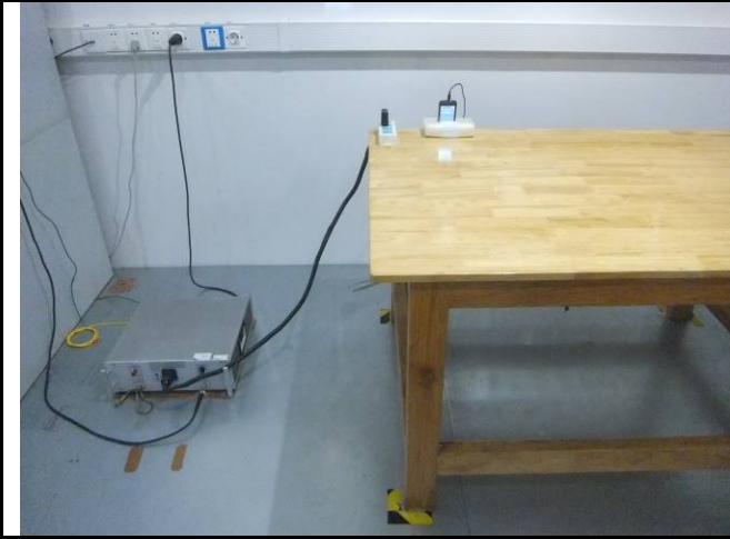
Conducted Emissions Test Setup Front View
