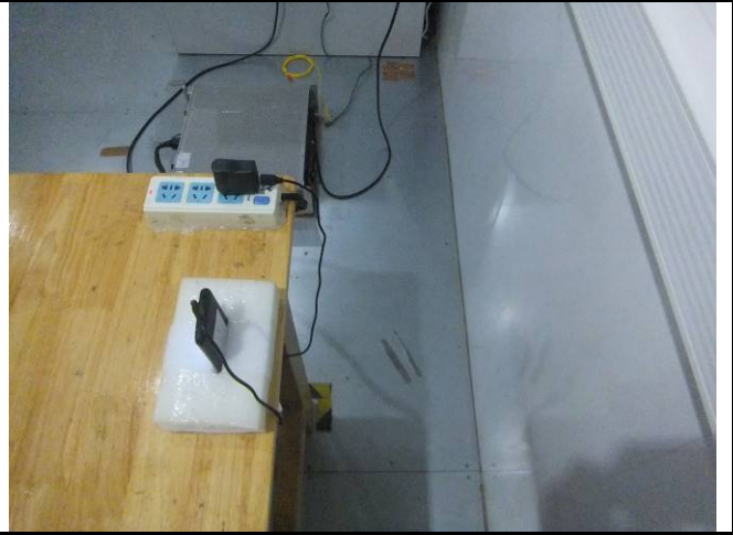
Conducted Emissions Test Setup Side View
