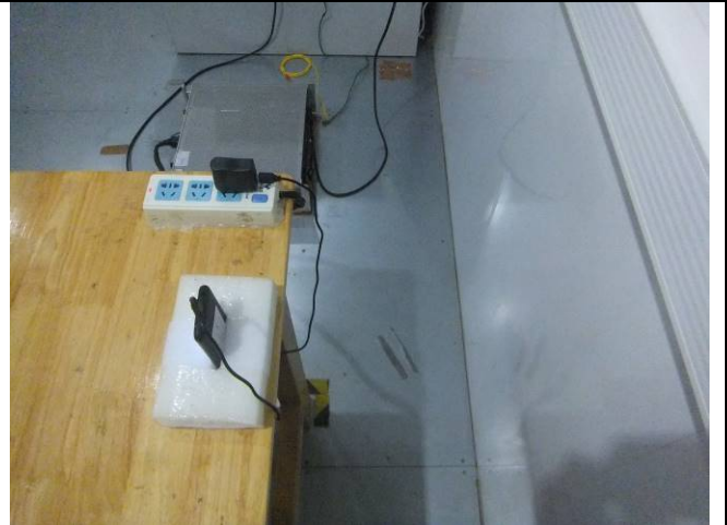
Conducted Emissions Test Setup Side View
