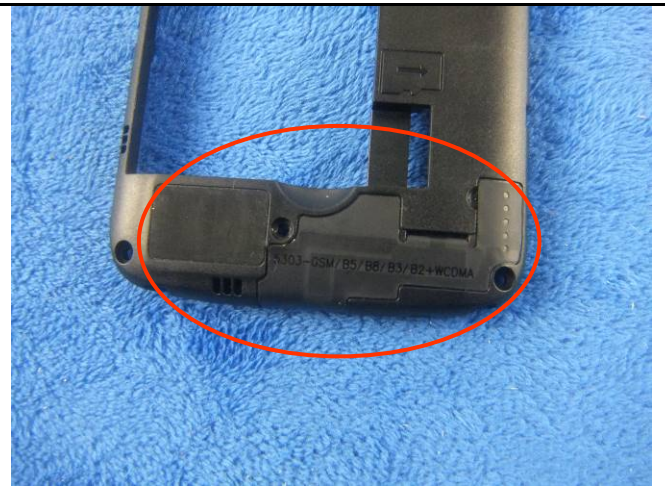
GSM/PC/S/UMTS-FDD Antenna View
