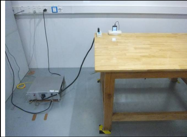
Conducted Emissions Test Setup Front View
