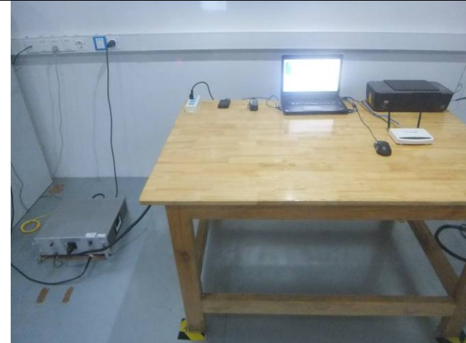
Conducted Emissions Test Setup – TF Card Front View
