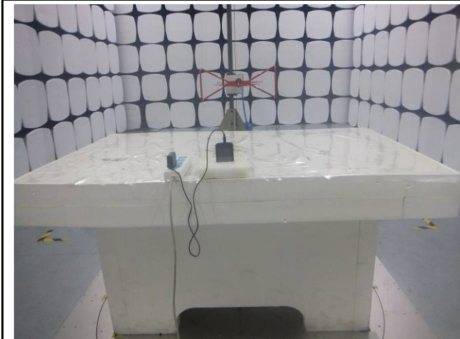
Conducted Emissions Test Setup Front View
