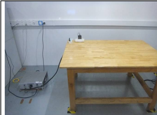
Conducted Emissions Test Setup Front View
