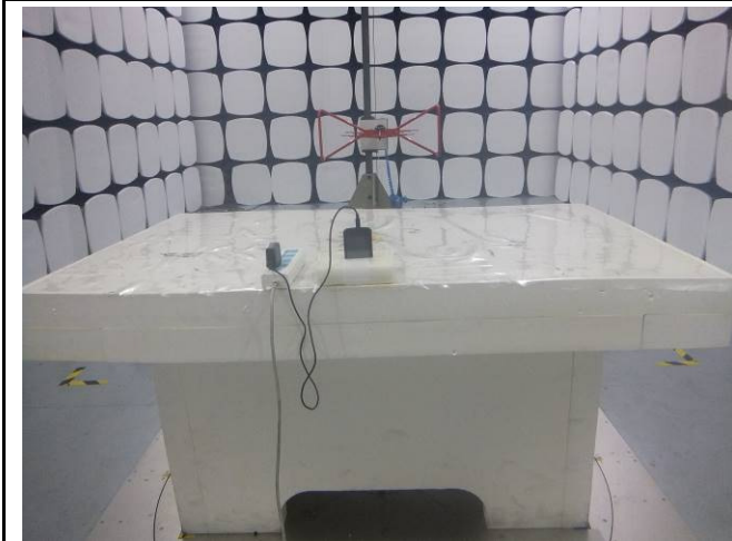
Conducted Emissions Test Setup Front View
