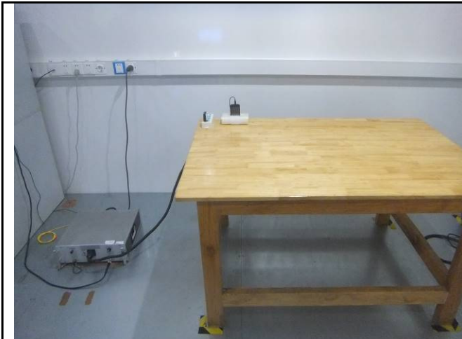
Conducted Emissions Test Setup Front View
