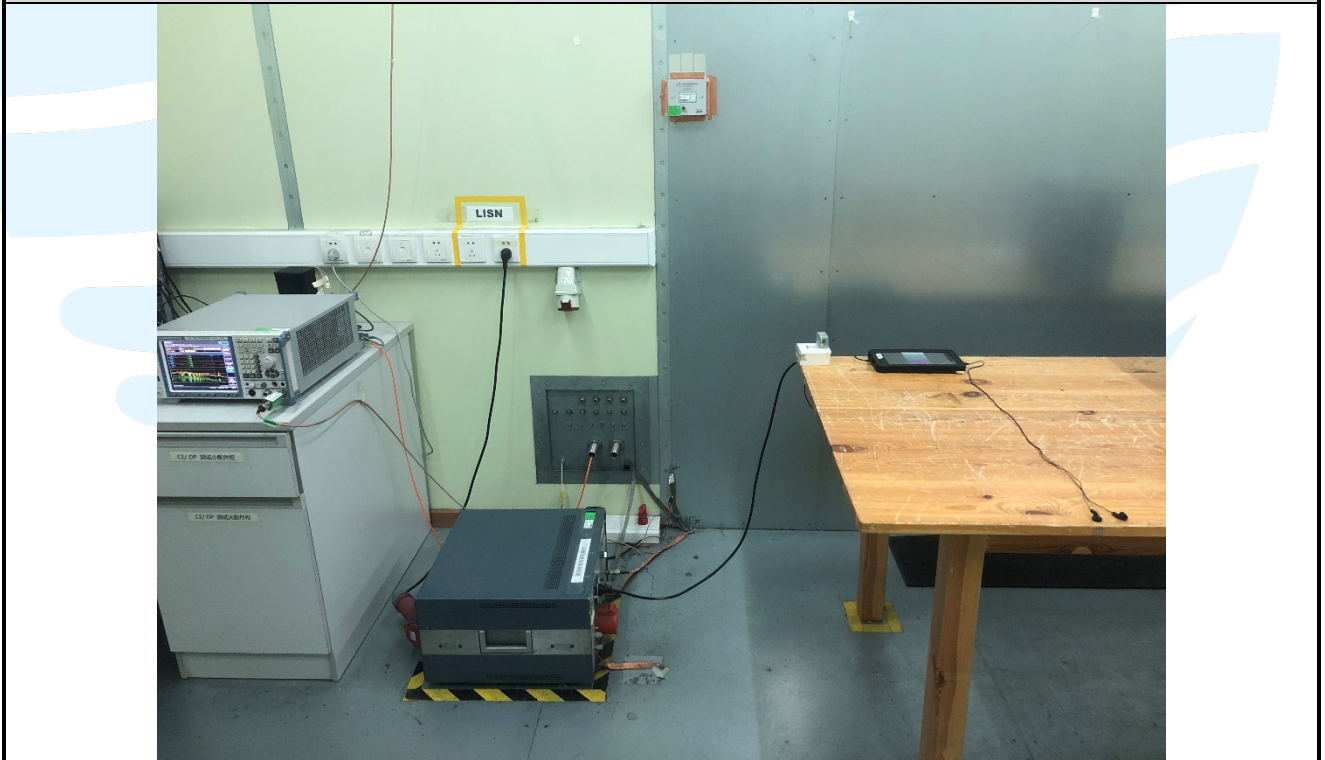
Conducted Emission Test Setup
