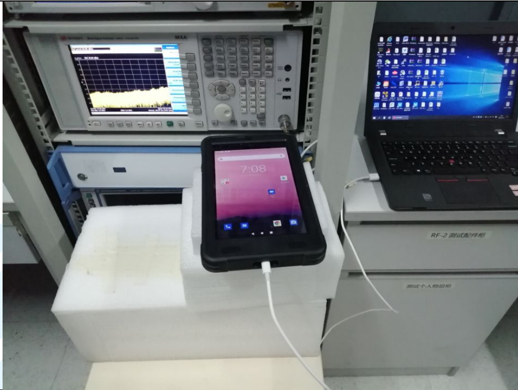
RF Conducted Test Setup
