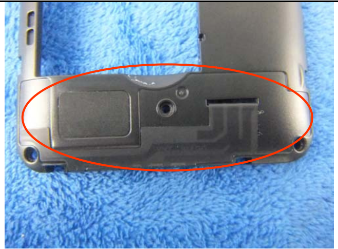
GSM/PCS/UMTS-FDD Antenna View
