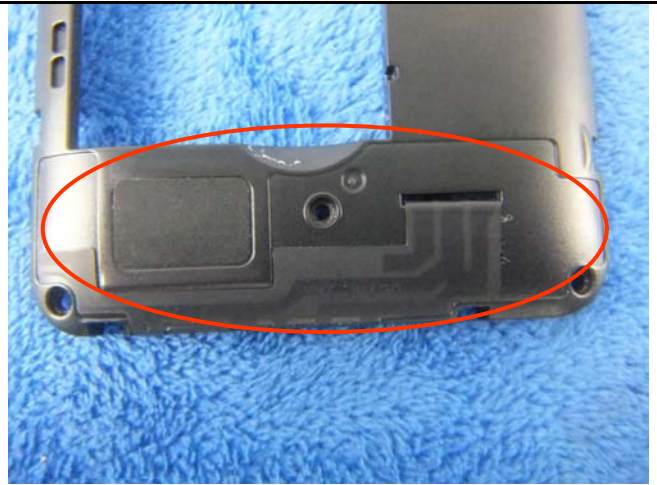
GSM/PCS/UMTS-FDD Antenna View
