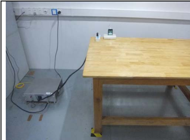
Conducted Emissions Test Setup Front View
