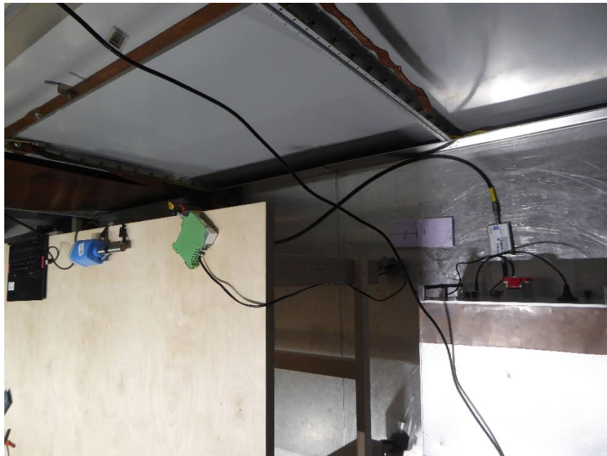
Test setup shielded room M4 Preliminary and final measurement 150 kHz – 30 MHz
