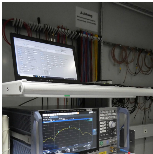
Test setup conducted @ antenna port Preliminary and final measurement 9 kHz – 26.5 GHz
