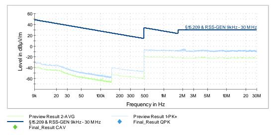
Remark: In the shown plot a distance correction factor was added to the measurement results to account for the different measuring distances according to standard (9 kHz to 490 kHz @ 300 m; 490 kHz to 30 MHz @ 30 m).
