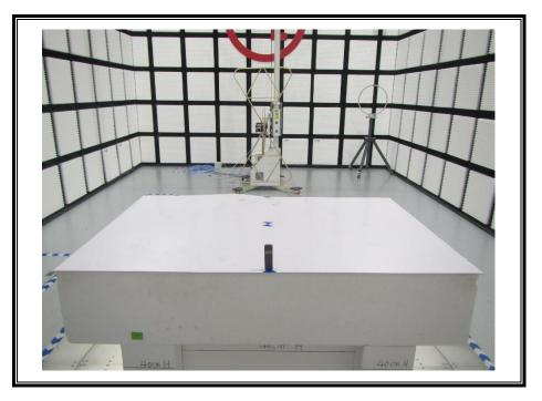
RADIATED RF MEASUREMENT SETUP (30MHz~1GHz)
