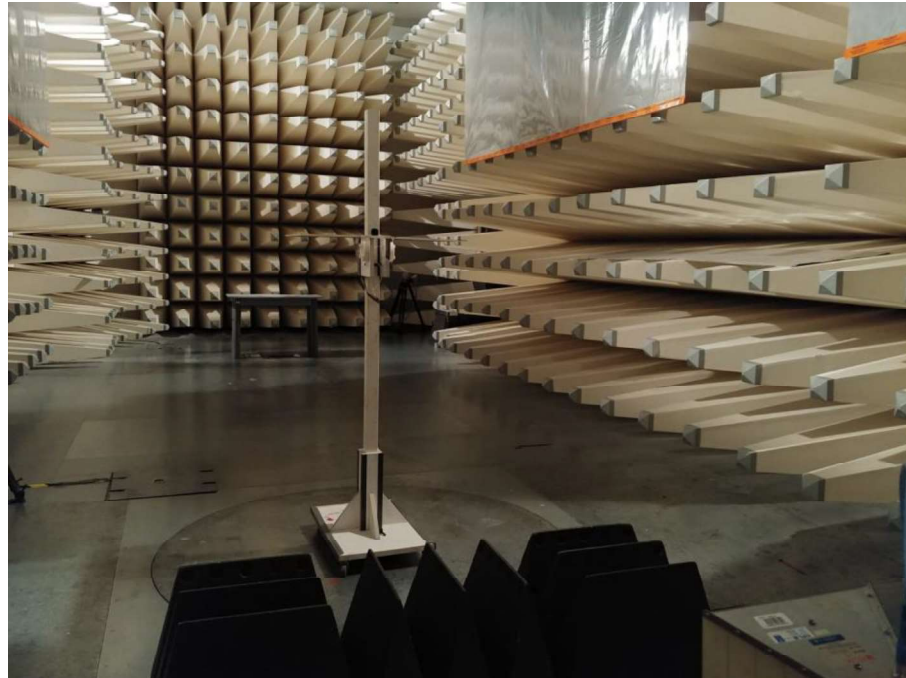
Set-up for Radiated Emission (above 1GHz)
