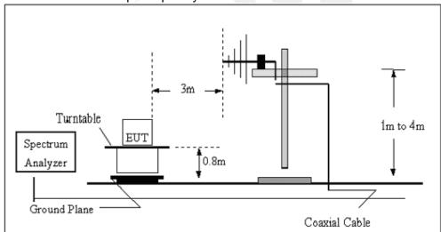
(C) Radiated Emission Test-Up Frequency Above 1GHz
