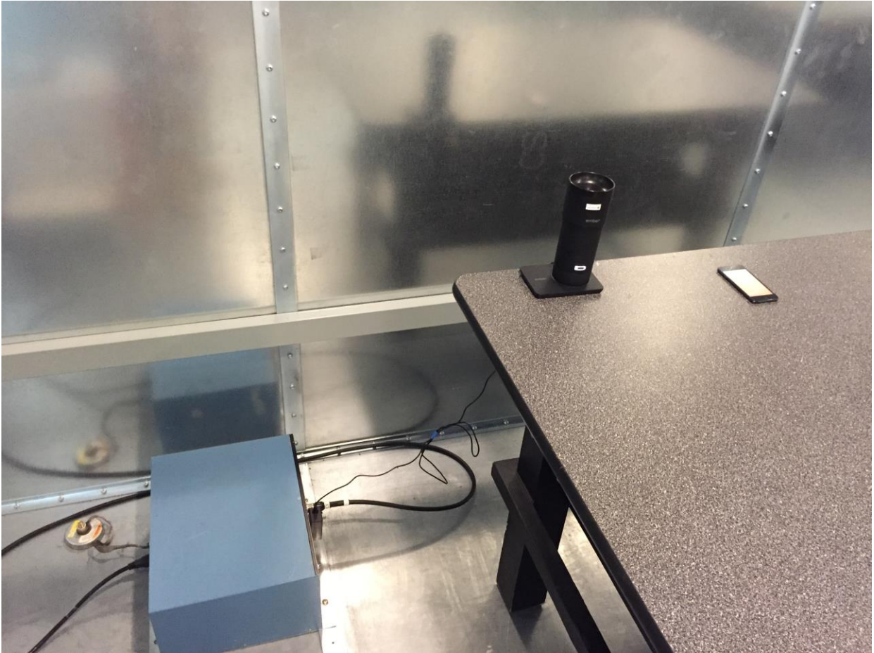
Figure 14: Conducted Emission Test Setup (Front)
