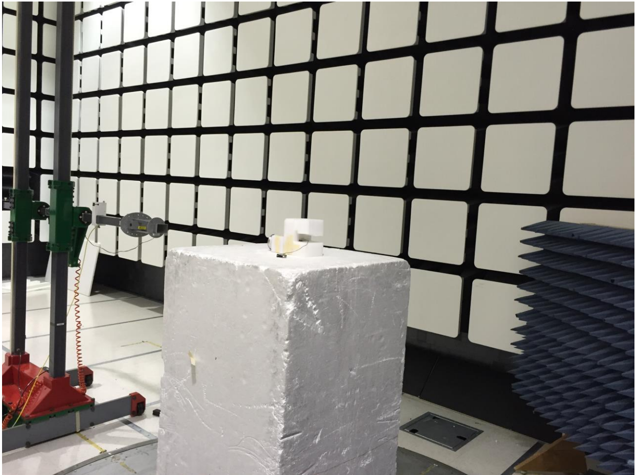
Figure 11: Test Setup for 18 GHz to 25GHz (Rear View)
