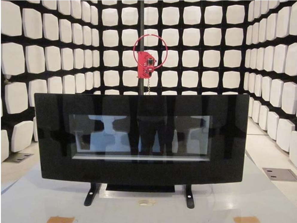
Measurement of Radiated Emission Test Set Up
