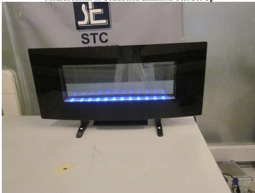
Measurement of Conducted Emission Test Set Up
