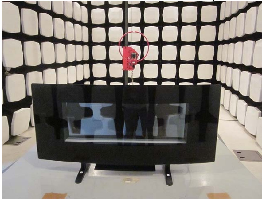
Measurement of Radiated Emission Test Set Up
