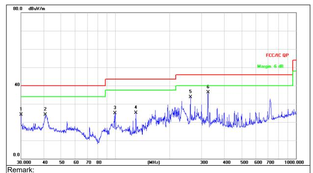
Factor = Antenna Factor + Cable Loss – Pre-amplifier.
