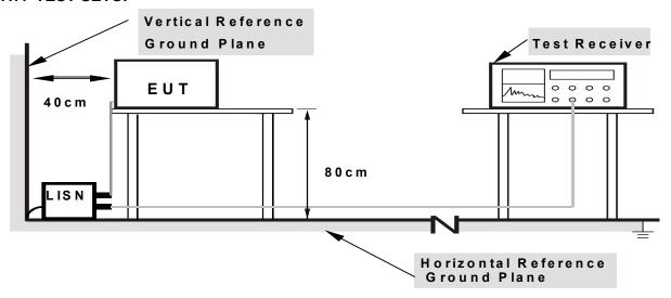
Note: 1.Support units were connected to second LISN. 2.Both of LISNs (AMN) are 80 cm from EUT and at least 80  $\,$
