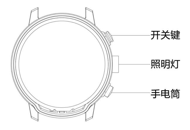
开关键: Switch button 照明灯: Light lens 手电筒: Torchlight button
