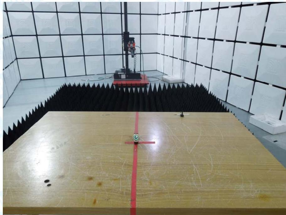
**Photo of Setup for Radiated Emission (Below 1 GHz)**
