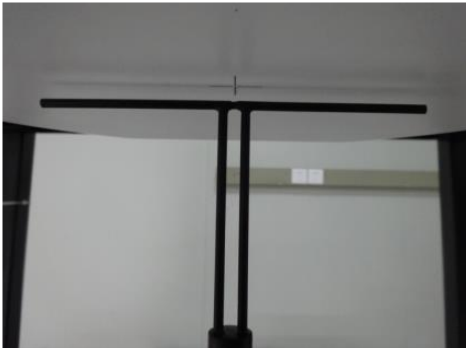
Photo of Dipole Setup
