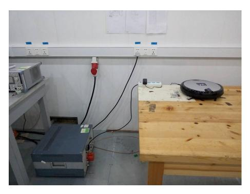
The EUT is placed in the 0.8 m high test table
