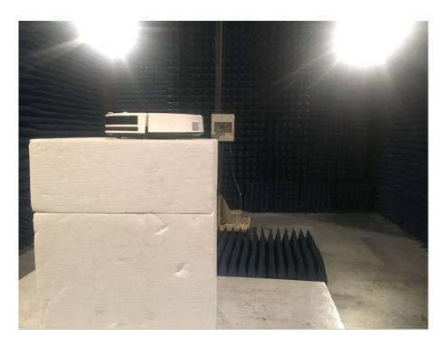
Above 1GHz: Test Height is 1.5m, the styrofoam block placed in the 0.8 m high test table
