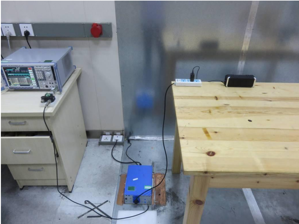
FCC RADIATED EMISSION TEST SETUP
