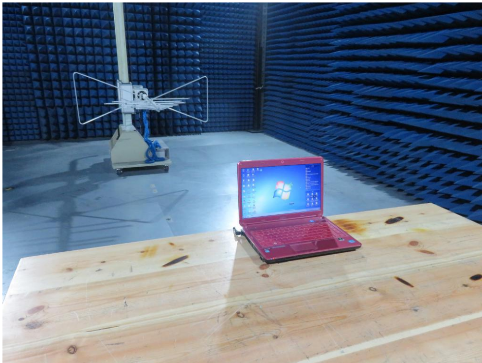
Photo of Radiation Emission Test
