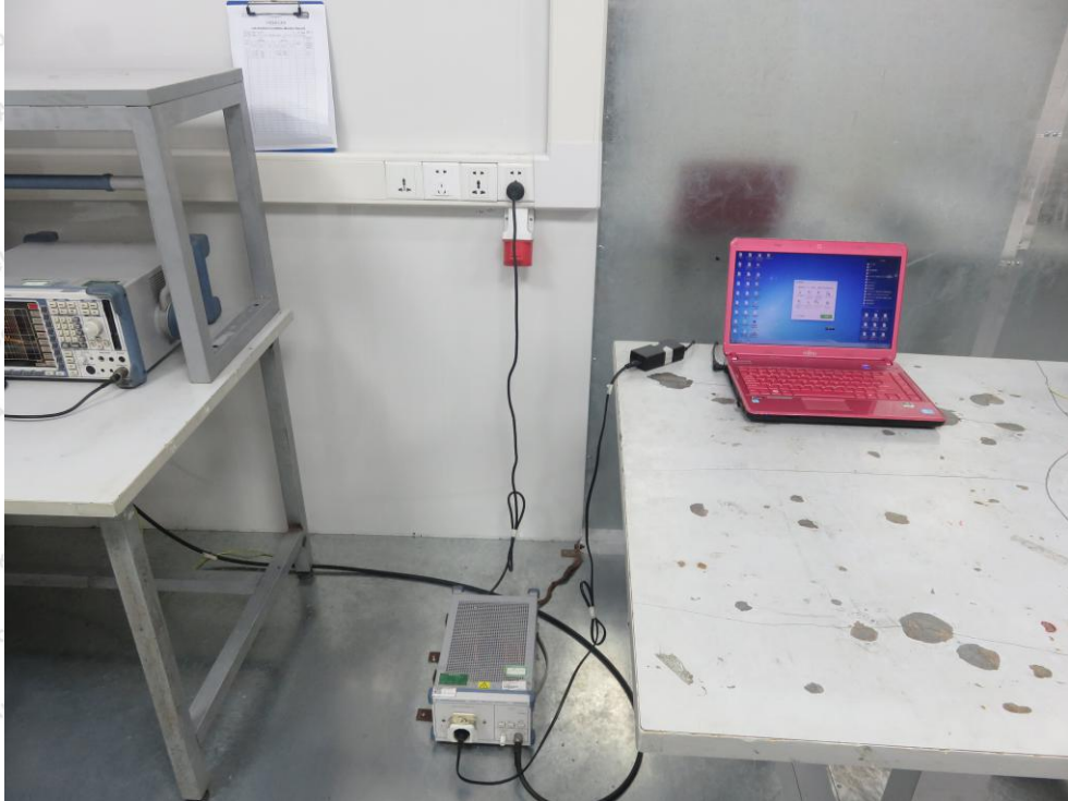
Photo of Conducted Emission Test
