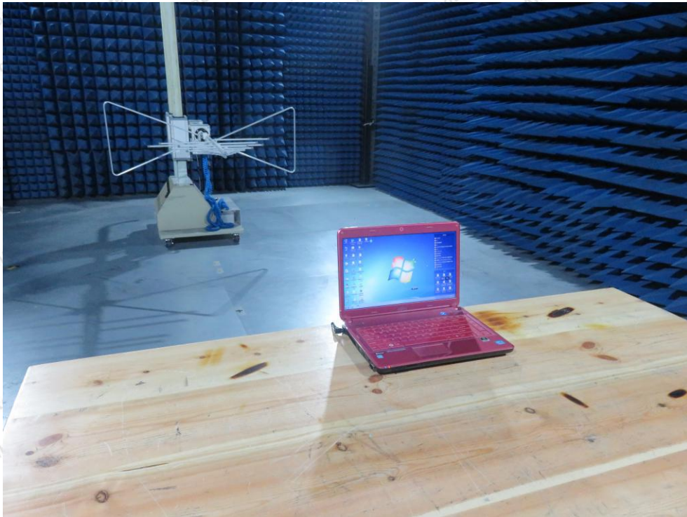
Photo of Radiation Emission Test
