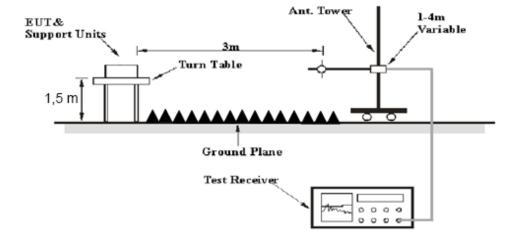
The radiated emission below 1GHz tests were performed in the 3 meters chamber test site A, above 1GHz tests were performed in the 3 meters chamber test site B, using the setup accordance with the ANSI C63.10-2013. The specification used was the FCC 15.209, and FCC 15.249 limits.
