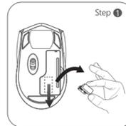
**EN** Fetch the wireless keyboard and mouse from the package, then fetch the USB receiver from the mouse battery compartment.
