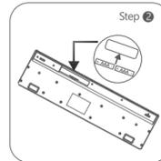
**EN** Put 2 AAA batteries into the keyboard in the right direction; Put 1 AA battery into the mouse in the right direction.
