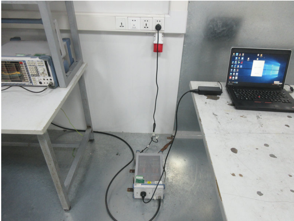
Photo of Conducted Emission Test
